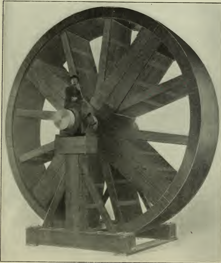
PULLEY 132 INCHES IN DIAMETER MADE IN TWENTY-EIGHT AND ONE-HALF HOURS
